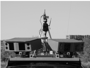
Fig. 1: Sensor configuration on a modified sport utility vehicle. The vehicle has 2 Ladars and a stereo pair of LWIR cameras.
