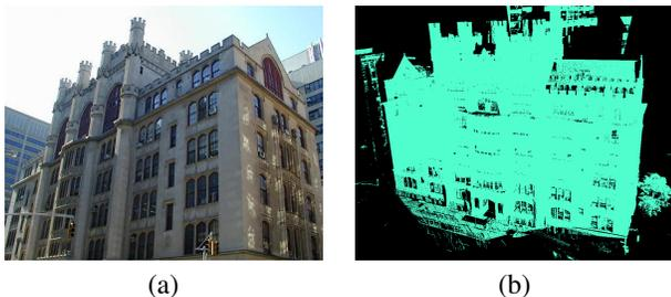
Fig. 3. (a) Input scene. (b) 3D point cloud of scene assembled by registering 14 scans, each having one million points.
