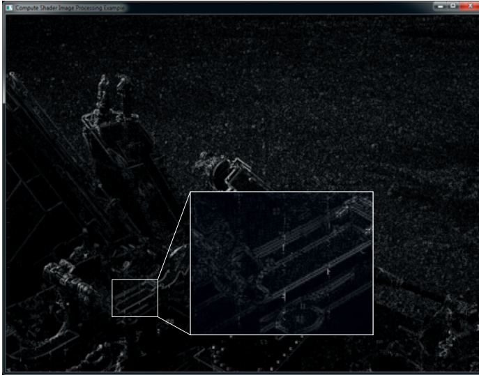
Figure 12.6 Image processing artifacts (Output of the image processing example, without barriers, showing artifacts.)
