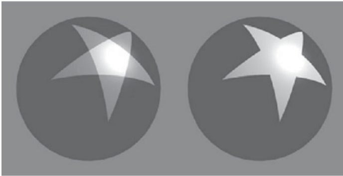
Figure 8.6 Intermediate results from “in” or “out” computation (Surface points that are “in” with respect to all five half-planes are shown in white, and points that are “in” with respect to four half-planes are shown in gray (A). The value of inorout is clamped to the range [0, 1] to produce the result shown in (B). (Courtesy of AMD.)
