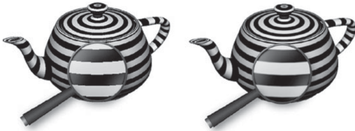
Figure 8.16 Effect of adaptive analytical antialiasing on striped teapots (On the left, the teapot is drawn with no antialiasing. On the right, the adaptive antialiasing shader is used. A small portion of the striped surface is magnified 200 percent to make it easier to see the difference.)
