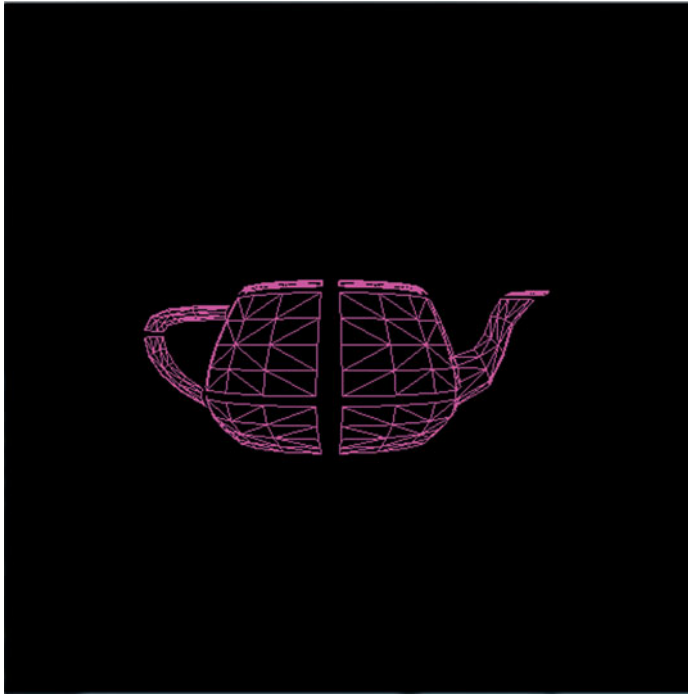
Figure 9.5 The tessellated patches of the teapot
