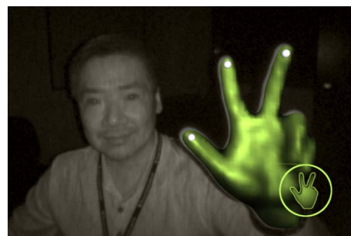
Figure 11: Gesture recognition using a 3D-TOF sensor.
