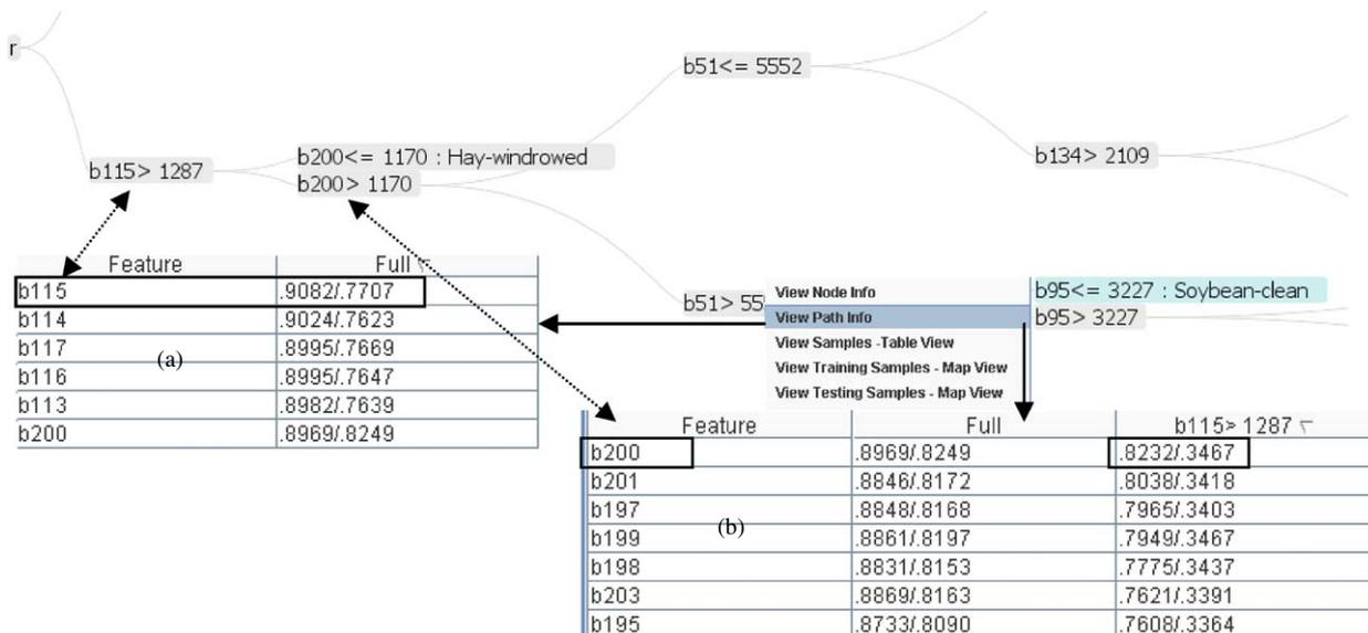
Fig. 3. Viewing and sorting information gain and gain ratio information from root to a selected node: understanding how partitioning attributes are chosen by decision tree classifier in VDM-RS. Subpanels: information gains and gain ratios for all the attributes using training samples under the root node (a) and node b115 > 1287 (b).
