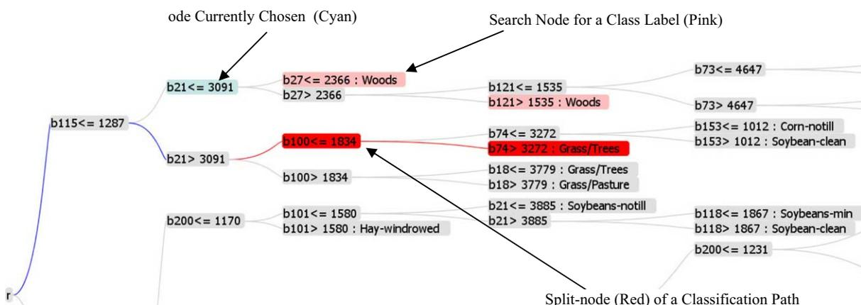
Fig. 2. Visualizing classification path of an individual sample in VDM-RS and identifying breaching point for an incorrectly classified sample. (For interpretation of the references to colour in this figure legend, the reader is referred to the web version of this article.)
