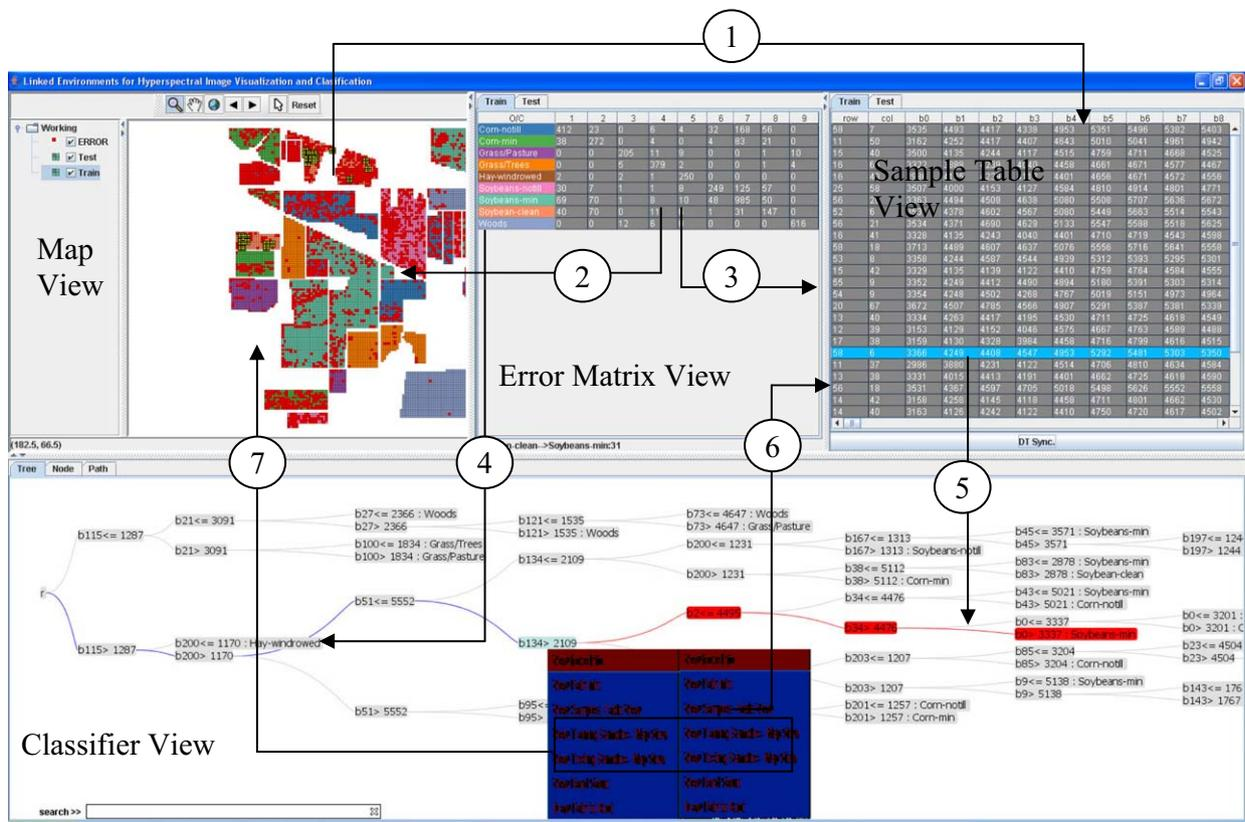
**Fig. 1.** Architecture, view components and coordination flows of VDM-RS. (For interpretation of the references to color in this figure legend, the reader is referred to the web version of this article.)
