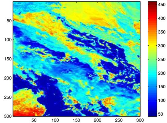
Figure 3. The image shown here is a  $300 \times 300$  pixel cropped section of SEVIRI Band 3 digital counts corresponding to the band 2 section shown in the previous image. The approach of the compression algorithm is to use a predict this image from the previous band 2 image.
