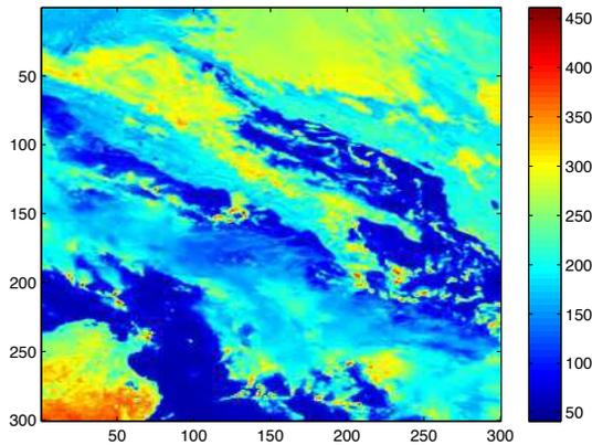
Figure 6. This shows the result of predicting SEVIRI band 3 by multiplying band 2 by the image in Fig. 5 after interpolating to using the a spatially varying linear predictor offset and linear scale factors applied to the values in band 2 using the per block linear predictor
