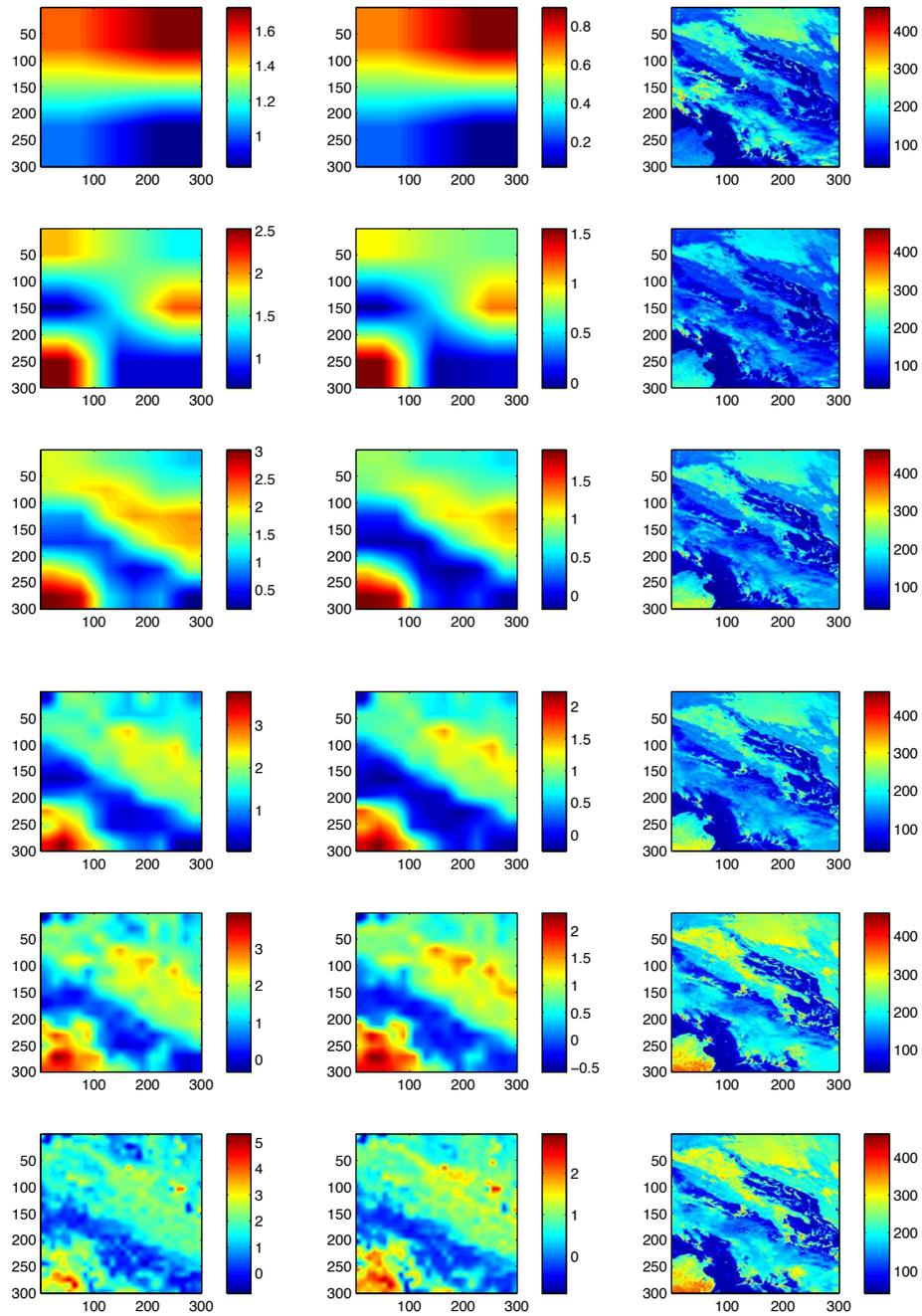
Figure 10. Each row shows the prediction model offset image, scale factor, and the predicted image computed for the same SEVIRI data shown in previous images. The window sizes used in the prediction are  $150 \times 150$ ,  $100 \times 100$ ,  $50 \times 50$ ,  $30 \times 30$ ,  $20 \times 20$ , and  $10 \times 10$ , from top to bottom row.
