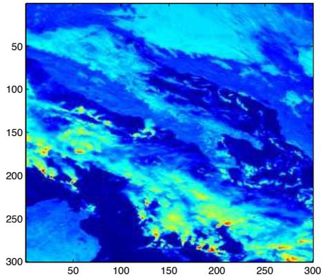
Figure 2. The image shown here is  $300 \times 300$  pixel cropped section of a SEVIRI Band 2 digital counts. Our algorithm actually operates on the whole image but to illustrate, we will assume that this cropped portion is the part of the data on which we will predict the a corresponding band 3 portion on. This band is compressed using conventional Jpeg2000 compression.
