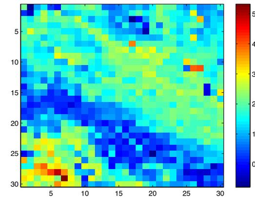
Figure 5. A  $30 \times 30$  image of prediction scale factors as determined by solving the least square linear regression as in the previous figure. The scale factor, like the offset, is computed during the *encoding* phase. The scale factor corresponds to the  $m$  in the per block linear predictor  $y = mx + b$ .
