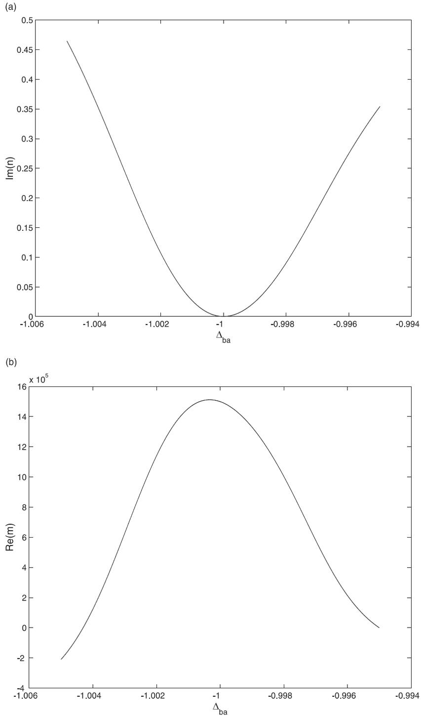
Fig. 1. The absorption coefficient and the group velocity reduction factor are plotted as function of the probe detuning in a driven optically dense cascade ladder three-level atom system.  $A_{cb} = 1$ ,  $\Omega_0 = 10^4$ ,  $\phi_{cb}^{\text{in}} = 0.1$ ,  $\alpha = 0$ .
