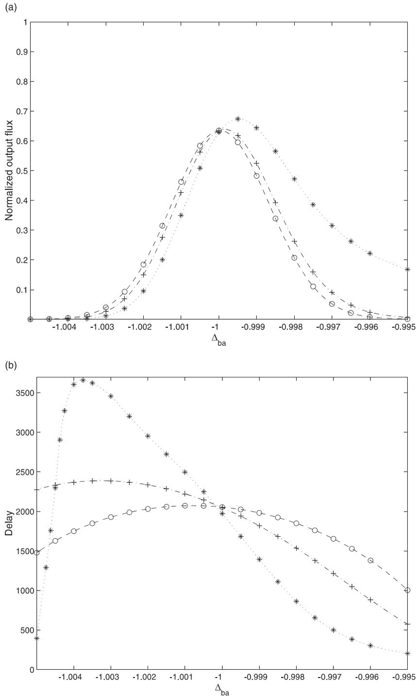
Fig. 3. The  $\varphi_{ba}$  probe field transmission coefficient and the pulse group delay for a driven dense ladder system having the following parameters:  $\Delta_{cb} = 1$ ,  $\Omega_0 = 10^4$ ,  $\varphi_{cb}^{\text{in}} = 0.1$ ,  $L = 2.25\lambda$ . The pump field is a cw field while the incoming probe field envelope is:  $\varphi_{ba}^{\text{in}}(\bar{z} = 0, \tau) = (0.001) \exp(-(\tau - 3000)^2/10^6)$   $\circ$ :  $\alpha = 0$ ;  $+$ :  $\alpha = 1$ ;  $*$ :  $\alpha = 4$ .
