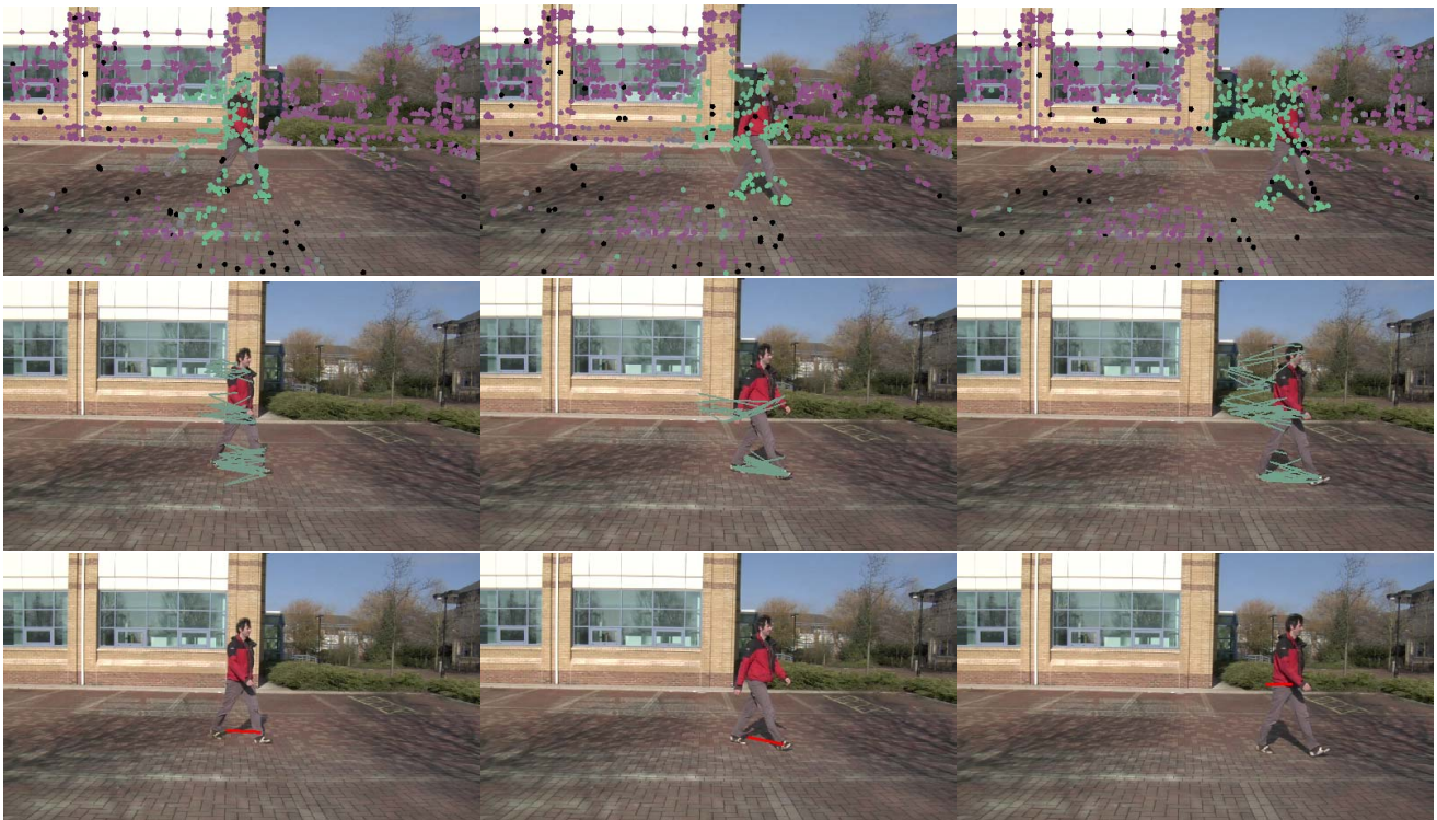
Figure 8. Results on Sequence II (showing a failure case). Feet are correctly detected in the first frames (left, middle), but in the last frame (right) a detection in the arm region occurs due to very similar motion. Top: Candidate points after the first stage are shown in green, rejected points in purple, points with short trajectories in black. Middle: Candidate pairs after the second stage are green line segments. Bottom: Final detection after running mean-shift.
