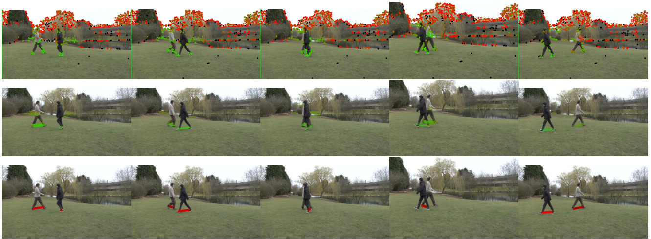
Figure 9. Results on Sequence III. Detection of two pedestrians walking across the scene from opposite directions. During the crossing phase only one pair of feet is detected, but subsequently two pairs are detected again. Top: Candidate points after the first stage are shown in green, rejected points in red, points with short trajectories in black. Middle: Candidate pairs after the second stage shown as green line segments. Bottom: Final detection result shown as red line segments.
