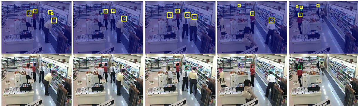
Figure 6. Frame #256, 266, 331, 505, and 936 of sequence [shopping mall]. The human head detections (top row) and our tracking results (bottom row).
