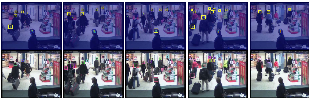
Figure 8. Frame #87, 204, 285, 774, and 980 of sequence [Airport CAM2]. The human head detections (top row) and our tracking results (bottom row).
