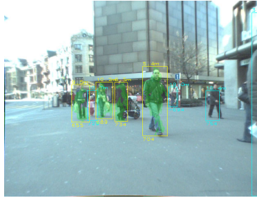
Fig. 7. Examples of detections (yellow boxes, with green overlay of segmented people) and misses (cyan boxes) for sequences from [26]. The false detection in the sequence 3 example is due to a reflection in the window.
