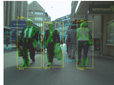
Fig. 8. Examples of detections (yellow boxes, with green overlay of segmented people) and misses (cyan boxes) for sequence 2 from [1]. There are false alarms on the car in the left image and the bus in the middle image. The misses are generally due to lack of stereo coverage or excessive clutter.
