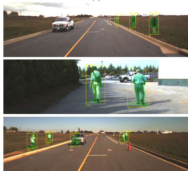
Fig. 3. (a) The performance resulting from 1000 trials of 80%/20% split cross-validation tests on 4,396 frames drawn from various scenarios. (b) Examples of images and detections from the various scenarios, with an example false alarm on the truck in the bottom image. The yellow boxes are detections, with a green overlay of the segmented person.
