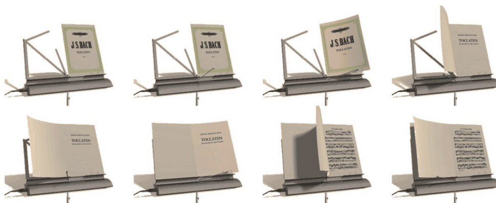
Fig. 3. Animation sequence of Volta Bene page turner.
