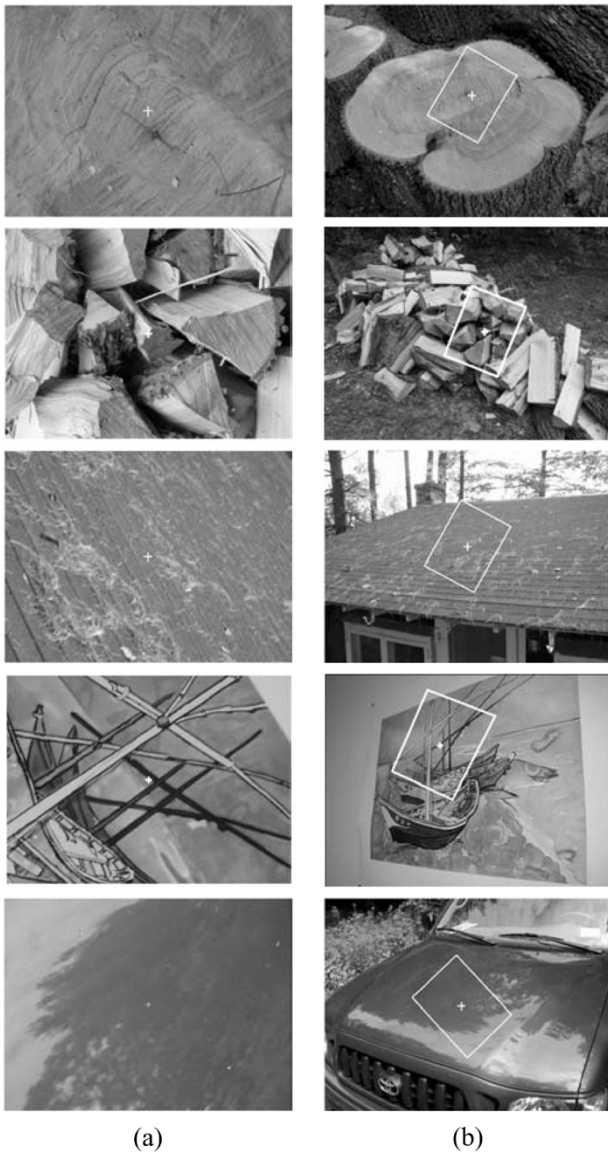
Fig. 8. (a) Observed images: 4 \times zoom, arbitrary rotation, and moderate perspective. (b) Registration results highlighted on reference images.
