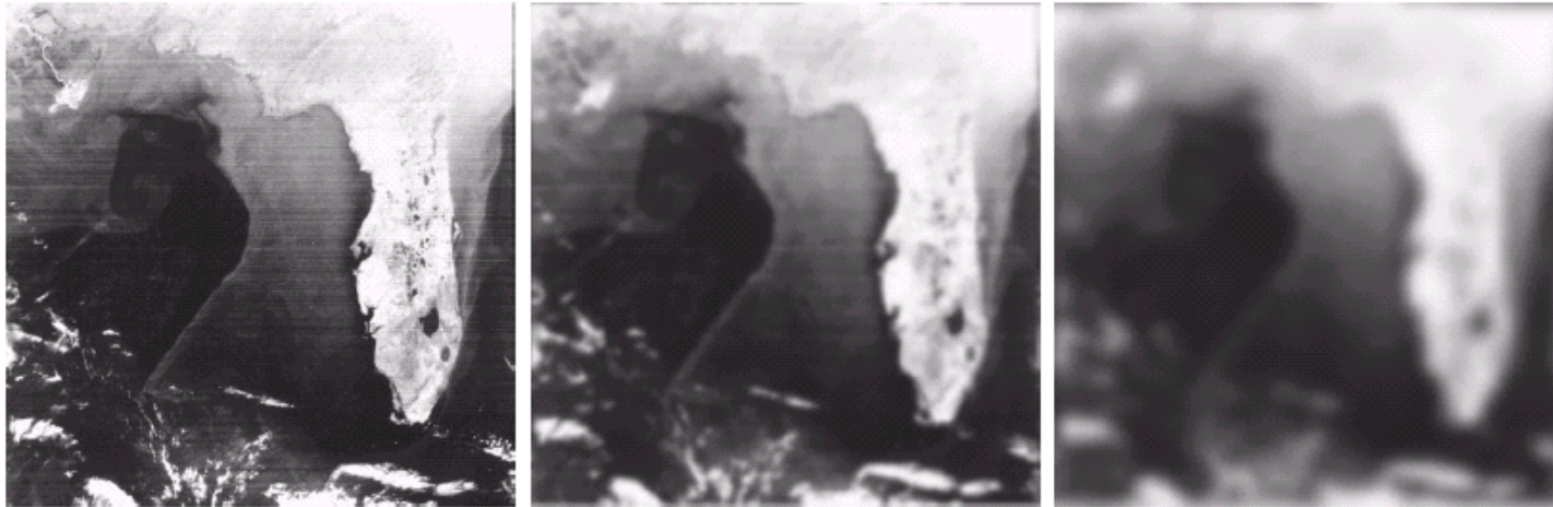
FIGURE 4.21 (a) Image showing prominent scan lines. (b) Result of using a GLPF with D_0 = 30 . (c) Result of using a GLPF with D_0 = 10 . (Original image courtesy of NOAA.)
