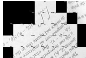
Figure 2: Feature blocks and displacement. Blocks with little or no structure in their texture are left out, to reduce the number of unreliable matches.
