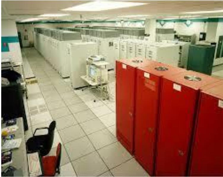
ASCI Red: 1997 First 1 Teraflops (sustained) system with 9298 Intel Pentium II Xeon processors (in 72 Cabinets)
